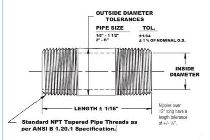
Steel Barrel Nipples with ASTM A733 Standard
