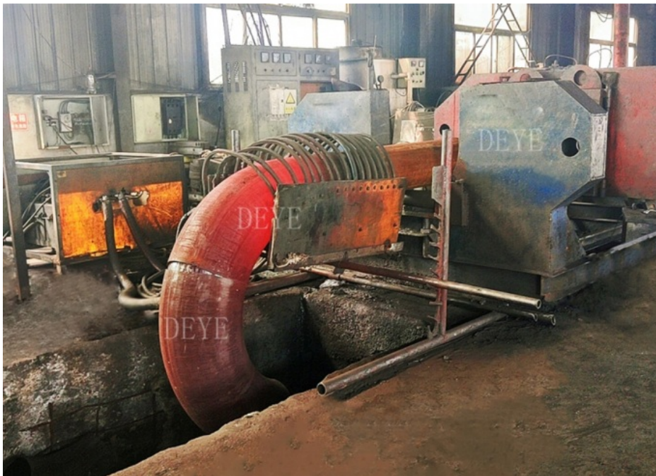
ELBOW Shaper Machining
