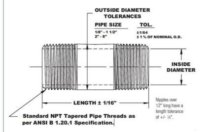
Steel Barrel Nipples with ASTM A733 Standard
