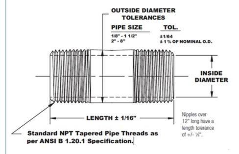
Steel Barrel Nipples with ASTM A733 Standard
